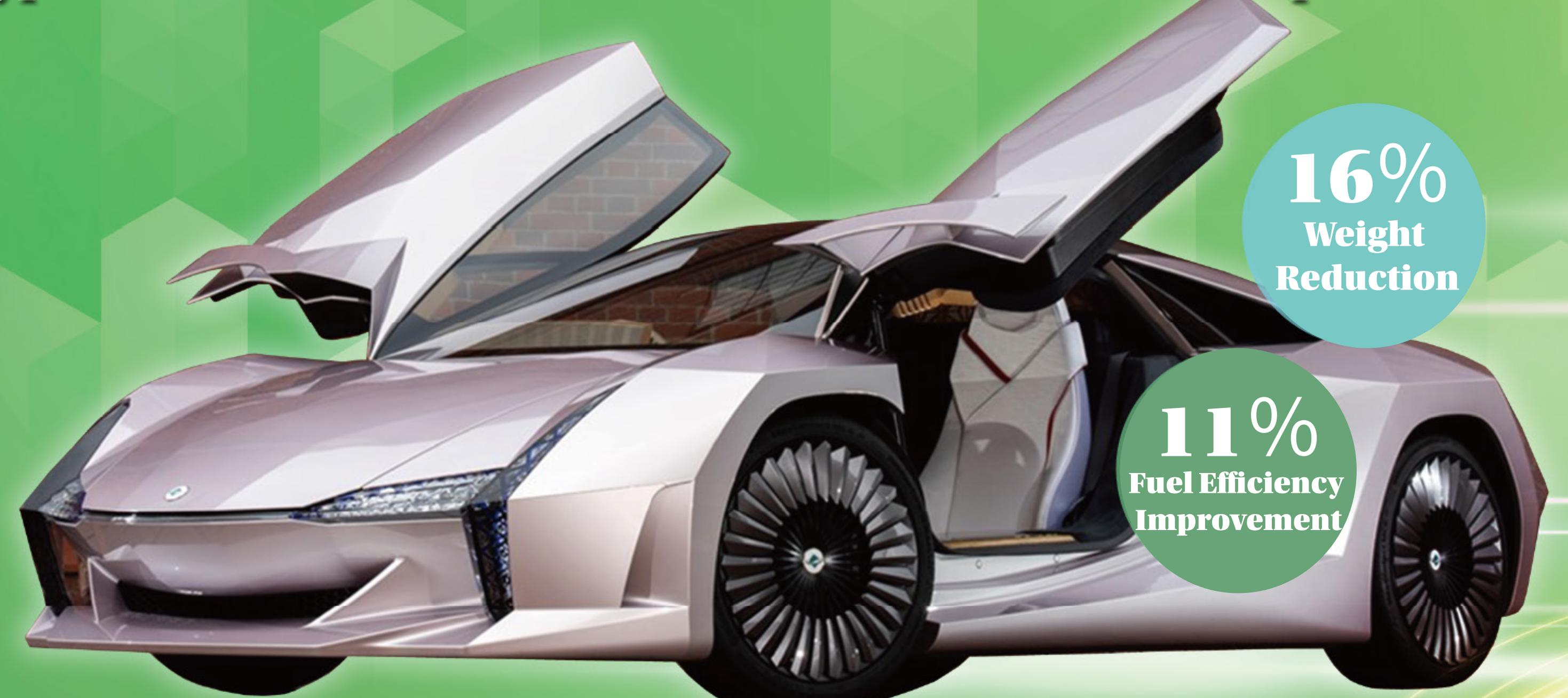
The NCV project applied CNF to 13 vehicle components, achieving a 16% weight reduction and an 11% improvement in fuel efficiency. This is a groundbreaking achievement showing that plant-derived CNF can reduce vehicle weight and improve future environmental performance.
